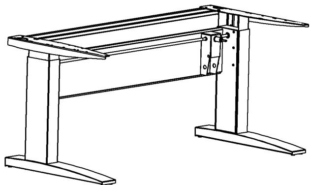
The left leg is connected to the front plate.
